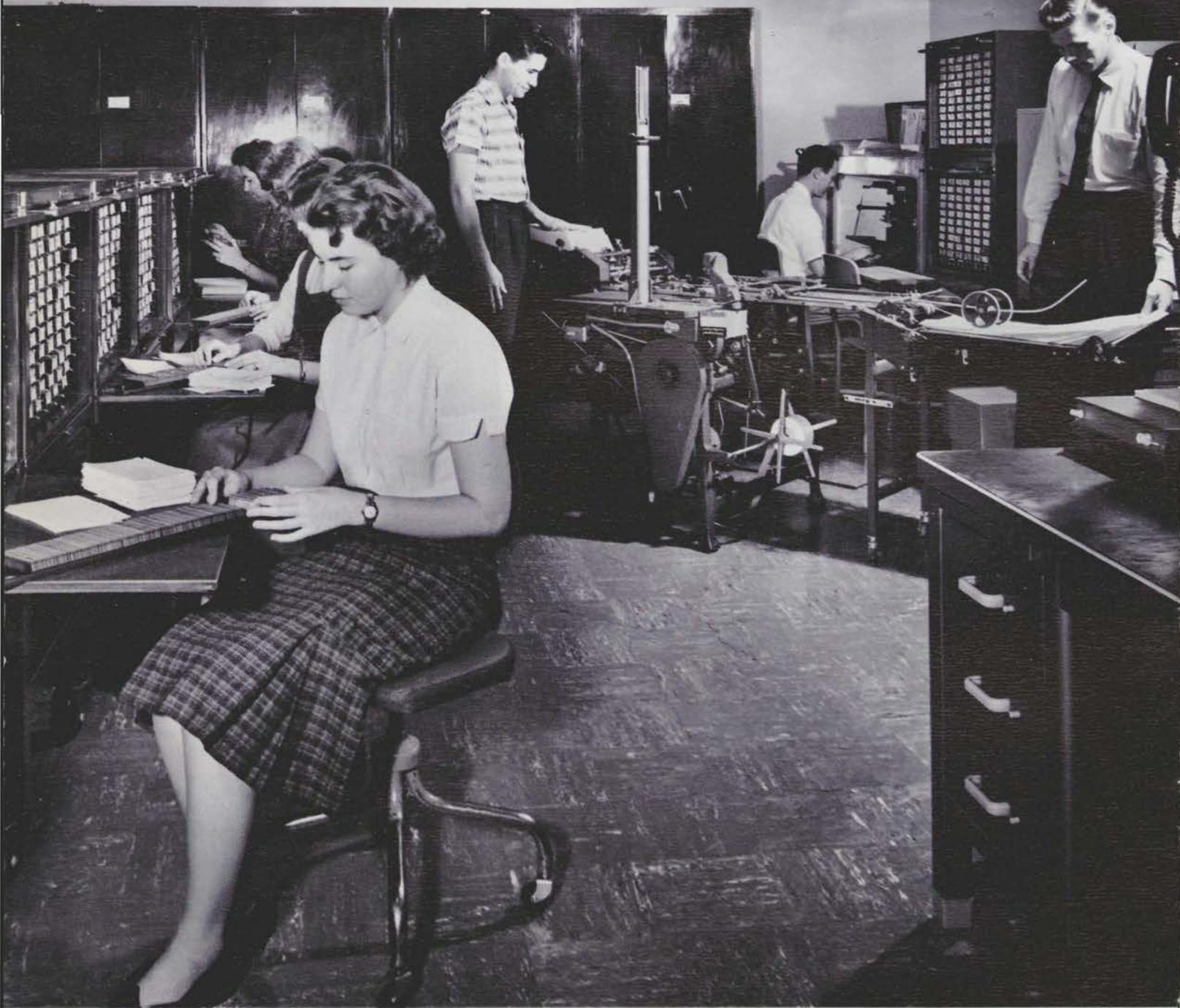
A faithful but outgrown system—Each of these cases contains seventy-seven trays of thin embossed metal name plates for printing the names and addresses directly on the Plain Truth. A new electronic system is gradually taking over the entire task of filing and addressing the magazines and bulletins.
