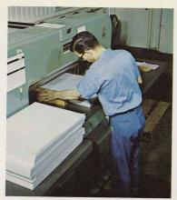
Del blocks a stack of paper in preparation for trimming with the Schimanek cutter.
